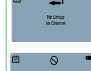
**Incorrect Channel** - This screen is to alert you that the QT Device is not on the correct channel or that the device is unable to communicate with the receiver.
